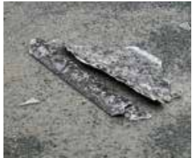
Non-friable asbestos may become friable after being damaged
