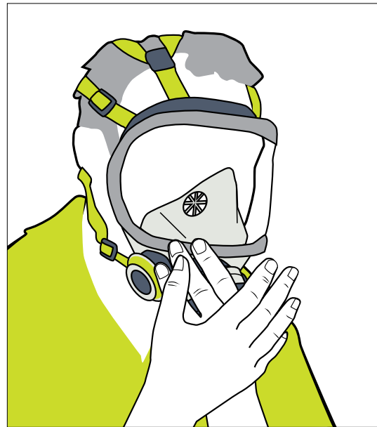
Figure 18: Conducting a fit check
